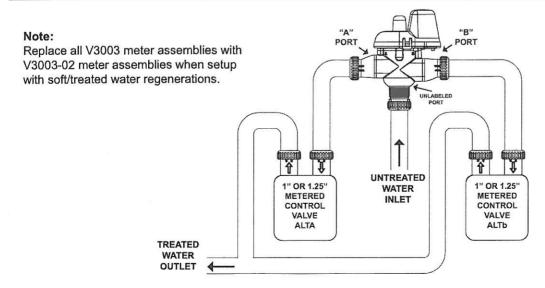
Motorized Alternating Valve & No Hard Water Bypass Valve Configurations
