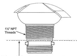
Quick Connect Nut Threads can be cut off to allow access to 1½" NPT Threads. Deburr and clean edge after cutting.
